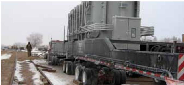
Charlie Creek's new transformer is loaded from the rail onto a truck at Belfield.
