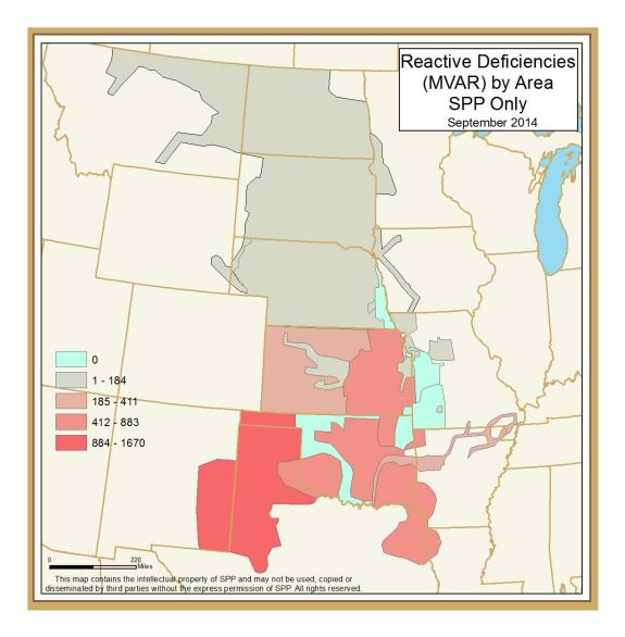
Figure 3: Transmission System Impact Analysis Part 1 - Reactive Deficiencies (MVAR)
