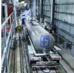
A truck is loaded with diesel exhaust fluid at the Great Plains Synfuels Plant.
