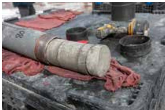
A core taken from the test well. These cores help geologists learn more about the rock deep below Wyoming's surface.
